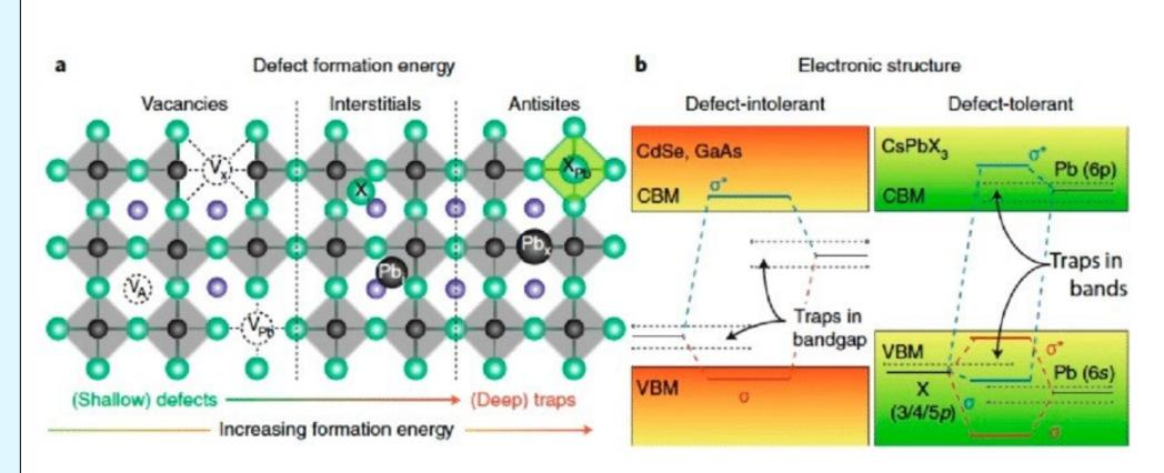
Semiconductor defect states are derived from different atomic orbitals. Depending on their location in the band structure of the host, the host exhibits different degree of tolerance to these defects. We investigate the fundamental defect physics of various semiconductors including hybrid perovskites for better understanding of their properties in device applications.
