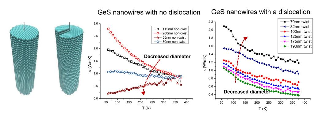
Abnormal thermal conduction in GeS nanowires with a single screw dislocation in the core. In twisted (dislocated) nanowires, thermal conductivity (*k*) shows unusual, opposite dependence on nanowire radius than that in normal nanowires. Dislocation core is found to host distinct atomic-scale structures and phonon properties. – *Liu et al, Publication in review (2024).*
