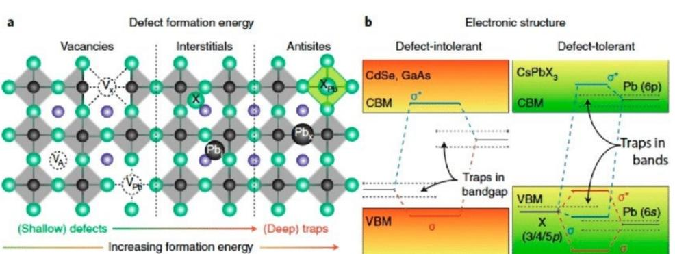
Semiconductor defect states are derived from different atomic orbitals. Depending on their location in the band structure of the host, the host exhibits different degree of tolerance to these defects. We investigate the fundamental defect physics of various semiconductors including hybrid perovskites for better understanding of their properties in device applications.
