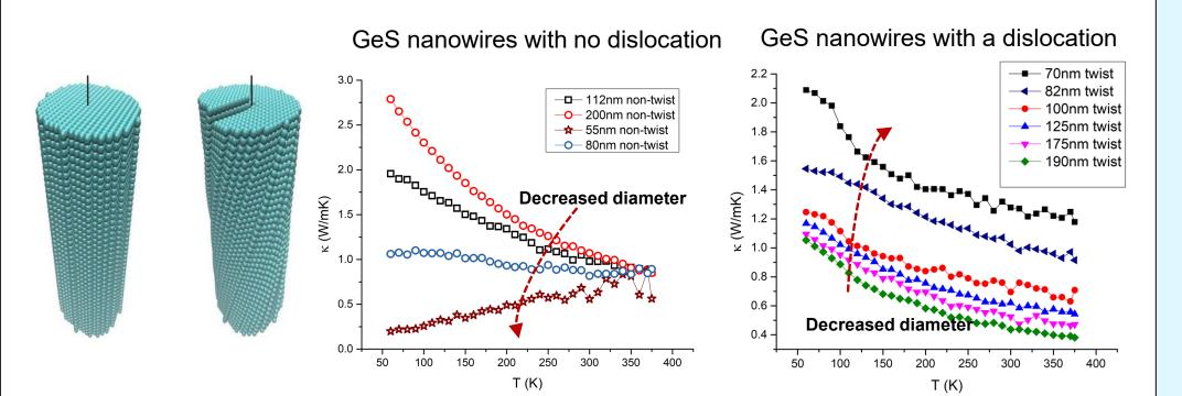
Abnormal thermal conduction in GeS nanowires with a single screw dislocation in the core. In twisted (dislocated) nanowires, thermal conductivity (k) shows unusual, opposite dependence on nanowire radius than that in normal nanowires. Dislocation core is found to host distinct atomic-scale structures and phonon properties. – Liu et al, Nature Materials (2025).
