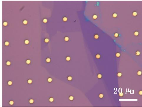
**Figure S1.** Optical image of BLG exfoliated onto an SiO<sub>2</sub>(300nm)/Si wafer with pre-etched holes.
