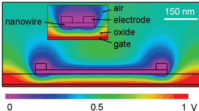
**Figure 4.** Electric potential distribution in the  $(y,z)$  plane in the BM model to show the potential variation along the NW due to the edge effect. In the simulation, the following parameters were used:  $R = 10$  nm,  $h = 50$  nm,  $L = 500$  nm (main) or 50 nm (inset),  $V_{\text{gate}} = 1.0$  V, oxide is  $\text{SiO}_2$ , and the electrodes have dimensions of 500 nm (length), 50 nm (height) and 50 nm (width) in  $x$ ,  $y$ , and  $z$  directions, respectively.
