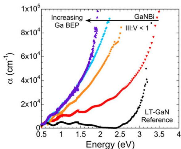
FIG. 2. Optical absorption spectra as a function of Ga BEP for a series of samples grown under similar Bi BEP and growth temperature. The circles represent the absorption spectra for a low-temperature molecular beam epitaxy (LT-MBE)-grown GaN film. As the Ga BEP increases, the incorporation of Bi into GaNBi increases until an RBS-determined III:V ratio of unity is reached for the left most spectra (triangles).
