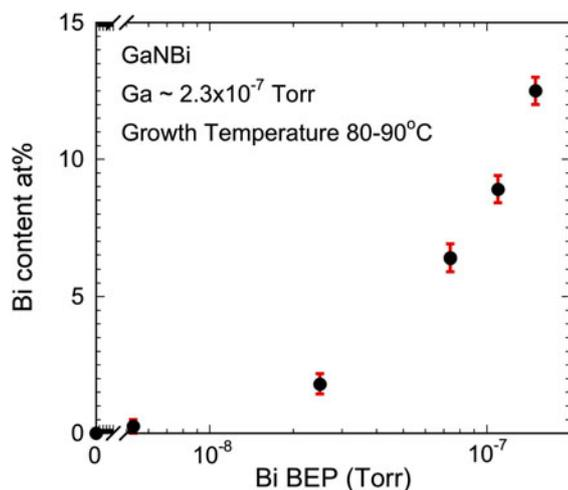
FIG. 3. The change in bismuth concentration as a function of Bi BEP. Even at high Bi at.%, the composition profile is uniform indicating minimal segregation of Bi to the surface.
