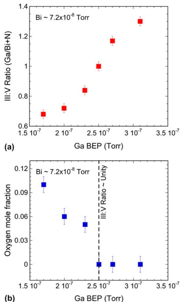
FIG. 1. (a) III:V ratio in GaNBi layers defined as the atomic concentration of Ga divided by the sum of the atomic concentration of Bi and N measured by Rutherford backscattering spectrometry (RBS), as a function of Ga beam equivalent pressure (BEP) during growth. (b) The oxygen content in the bulk of the film as determined by resonance RBS. Note that oxygen incorporation is suppressed when RBS-determined III:V is  $\sim 1$ .
