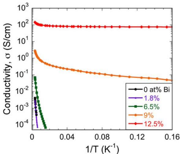
FIG. 5. Temperature dependence of the conductivity of GaNBi with varying Bi contents. The room temperature conductivity increases and the conductivity temperature dependence decreases with increasing Bi content.
