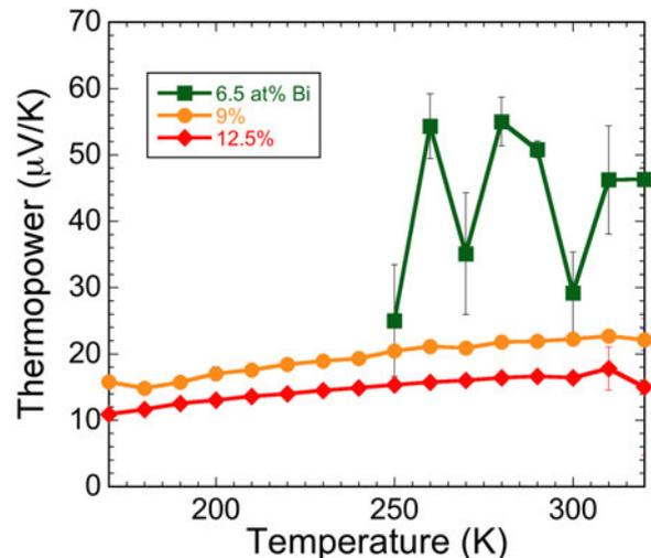
FIG. 6. Temperature dependence of the thermopower of GaNBi with varying Bi contents. The positive value indicates that holes are the majority carrier. The data for the sample with 6.5 at.% Bi has more variation due to the higher resistance of the sample.
