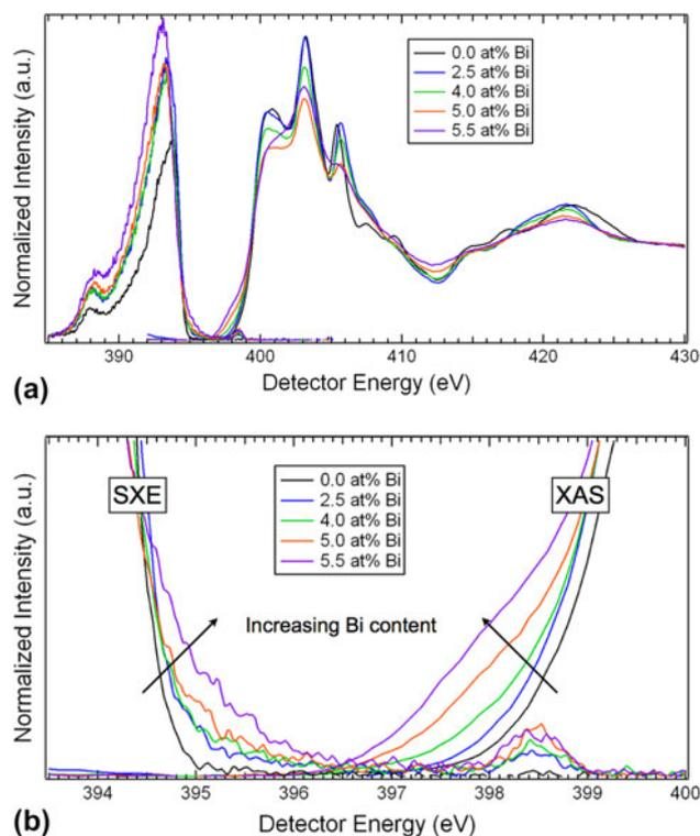
FIG. 7. (a) The nitrogen  $K$ -edge soft x-ray emission (SXE) spectroscopy (left side) and total fluorescence yield x-ray absorption spectroscopy (XAS) (right side) of GaNBi films with various Bi contents. The threshold-excited elastic emission peak near 398.5 eV was used to align the SXE spectra to the XAS. (b) Magnified view of the SXE and XAS of GaNBi with various Bi contents highlighting the changes to the band edge positions.
